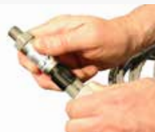
Cables are prefabricated and snap onto sensors with industrial deutsch connectors. This eliminates wire twisting when tightening sensors. IP65 rated for outdoor use when
